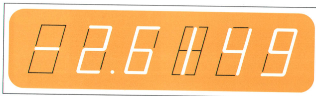
Fig. 3. Displayed characters are generated by modulating these figures. The digit 1 is shifted to the center of the pattern.
